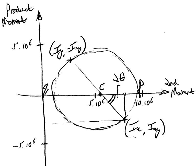
P axis is  $23.54^\circ$  anticlockwise from the x-axis
